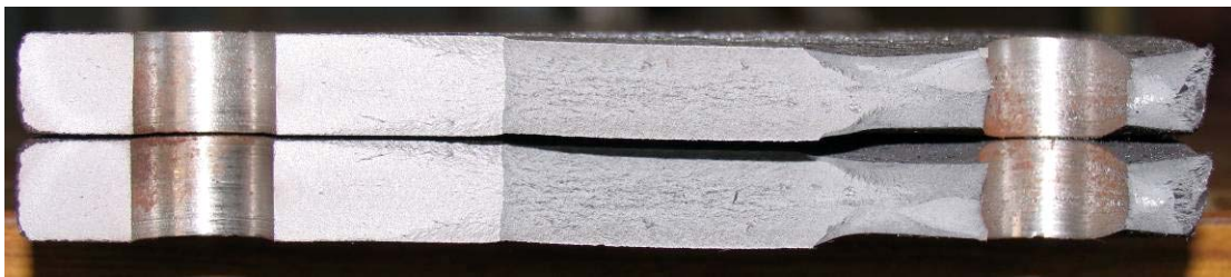
Figure G.9: Cross-Section of A36 - Punched Hole Plate Specimen at Failure, 11/16 in. Holes, Normal Die Size, N=768,176
