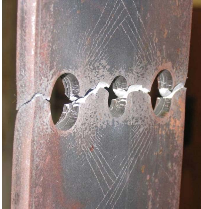
Figure 4.4: Reduced Net Area Plate Specimen Failure – Punched Holes
