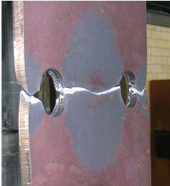
Figure 4.2: Typical Failed Punched Hole Plate Specimen
