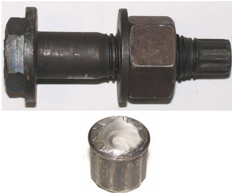
Figure 3.33: 7/8 in. A490 Twist-Off Type Bolt Used for Tests
