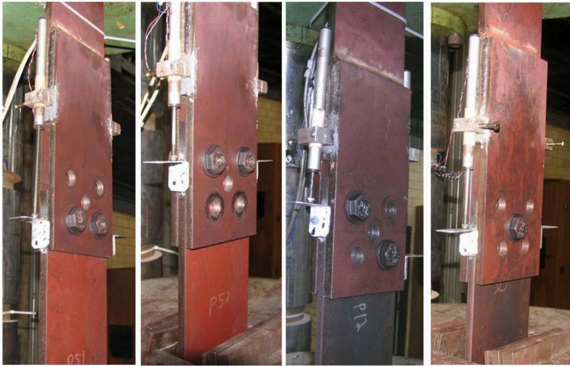
Figure 3.30: Orientations of Test Specimens in Pull Assembly
