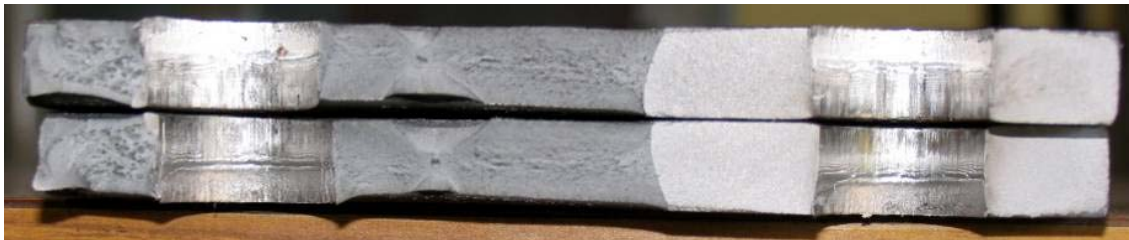
Figure G.4: Cross-Section of A572 Grade 50 - Punched Hole Plate Specimen at Failure, Normal Size Die, N=550,643
