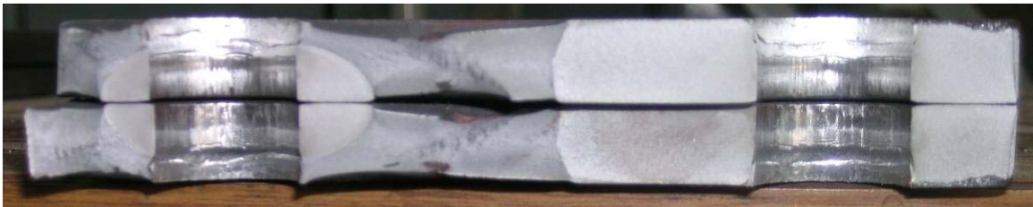
Figure G.8: Cross-Section of A588 - Punched Hole Plate Specimen at Failure, Normal Die Size, N=431,073
