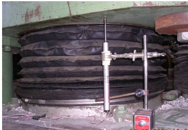
Figure 3.24: Linear Potentiometer at Base of UTM
