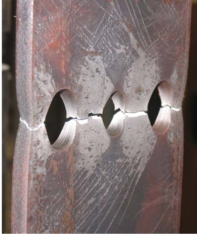
Figure 4.3: Reduced Net Area Plate Specimen Failure – Drilled Holes
