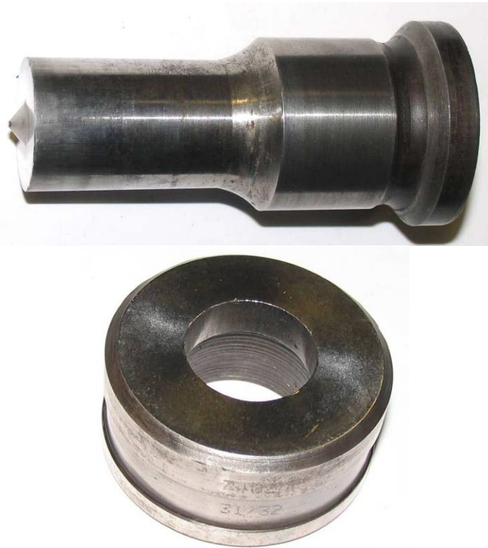
Figure 3.18: 15/16 in. Punch with 31/32 in. Die (At End of Testing)
