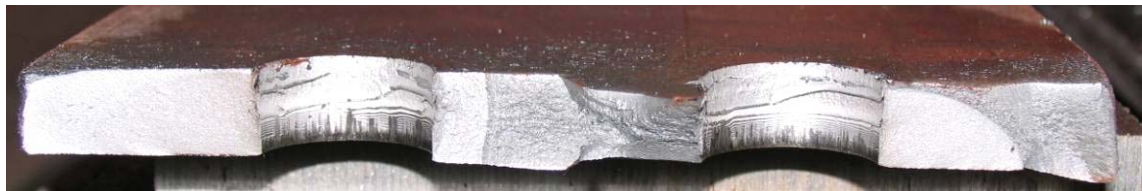
Figure G.13: Cross-Section of A36 - Punched Hole Plate Specimen at Failure, Larger Edge Distance, Normal Die Size, N=690,426
