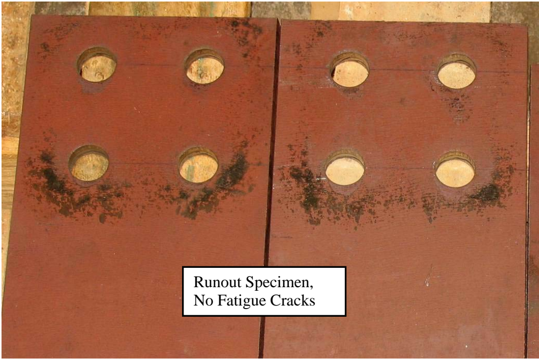
Figure G.15: Typical Pretensioned Bolt Connection Fatigue Runout Specimen Surfaces, at End of Testing
