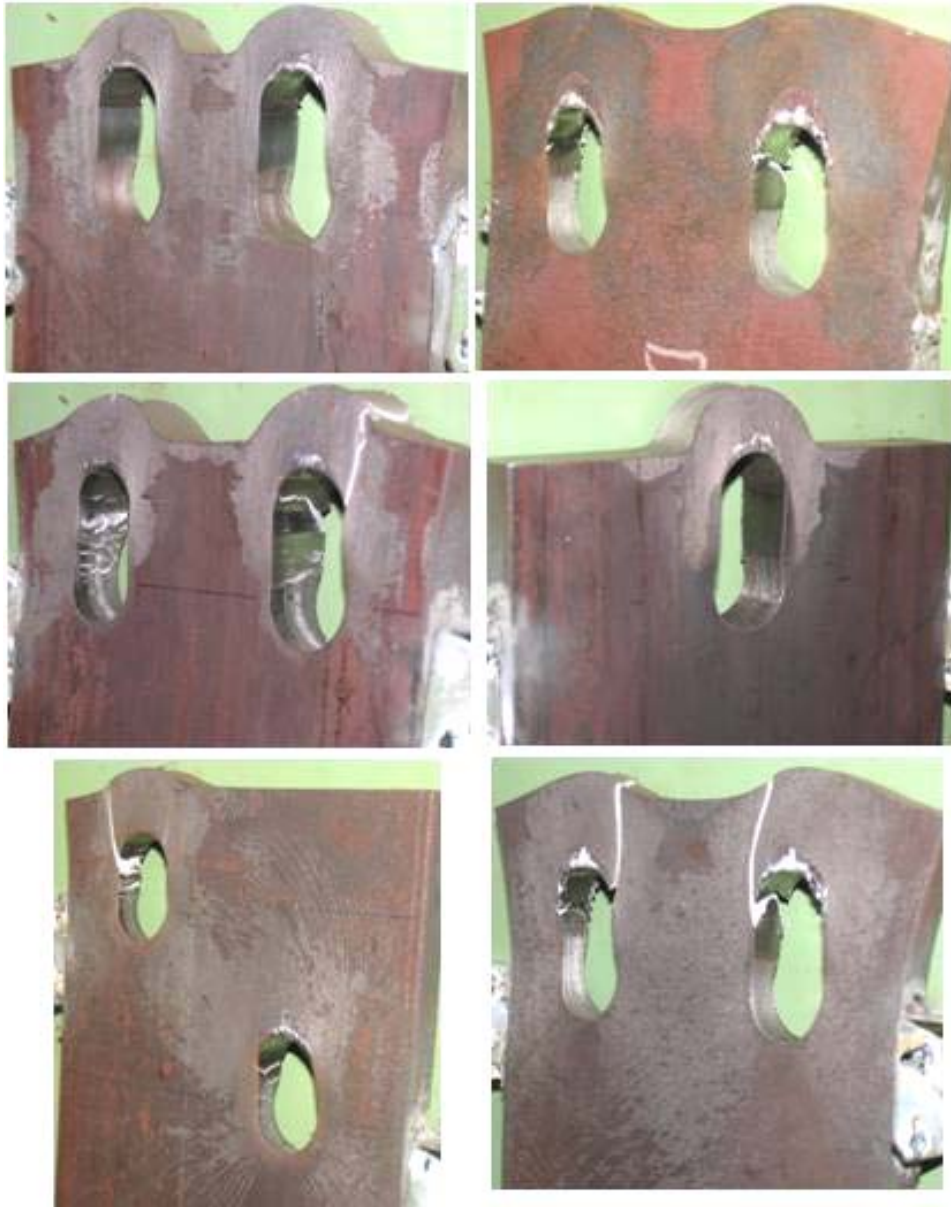
Figure 4.21: Experimental Bearing Type Failures
