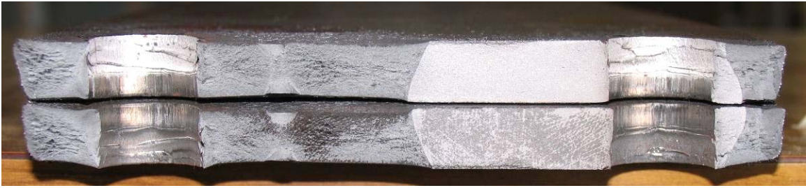
Figure G.11: Cross-Section of A36 - Punched Hole Plate Specimen at Failure, 13/16 in. Holes, Normal Die Size, N=662,744
