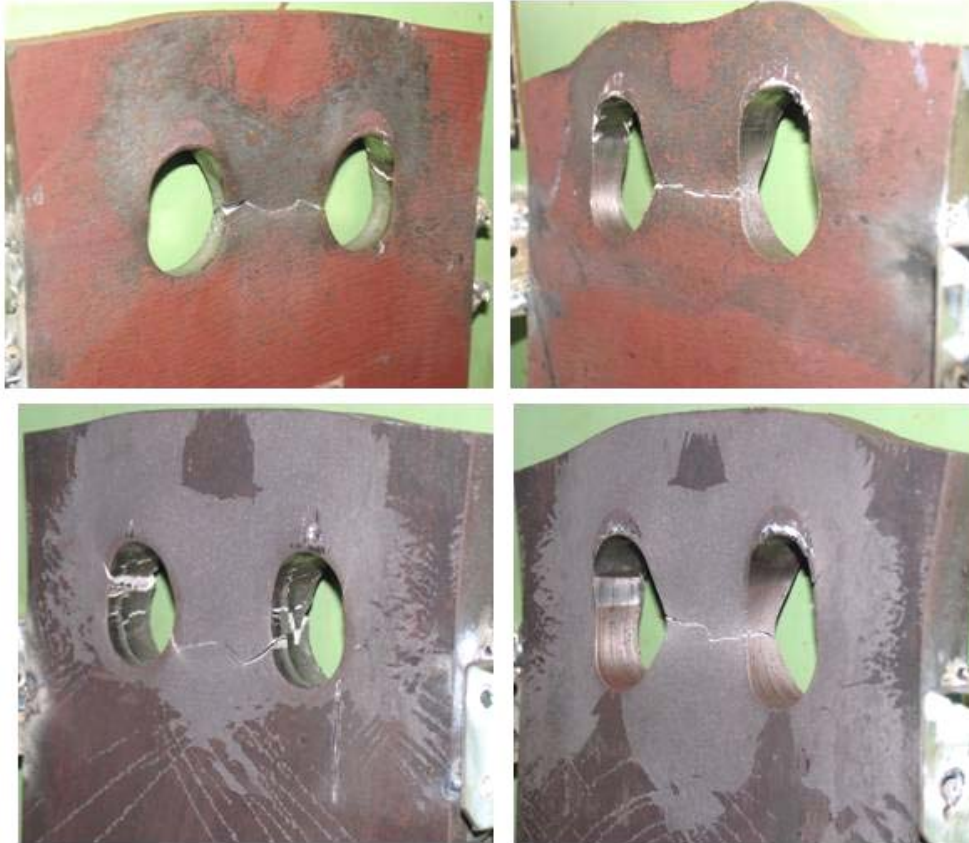
Figure 4.20: Experimental Block Shear Type Failures
