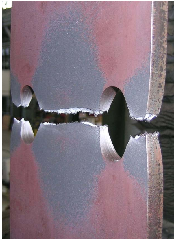
Figure 4.1: Typical Failed Drilled Hole Plate Specimen
