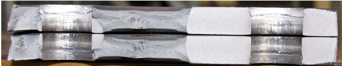
Figure G.7: Cross-Section of A588 - Punched Hole Plate Specimen at Failure, Normal Die Size, N=414,480
