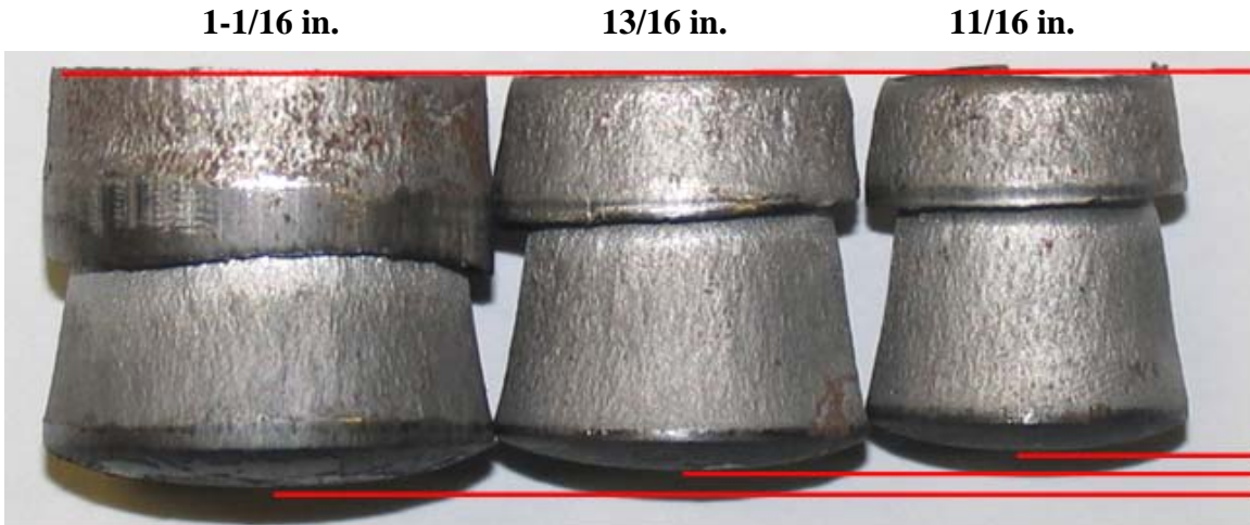
Figure A.1: Punched Hole Slugs in 1 in. Thick Plate
