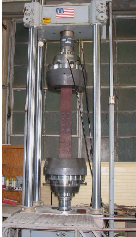
Figure 3.25: FSEL 220-kip MTS Load Frame, Shown with Connection Specimen
