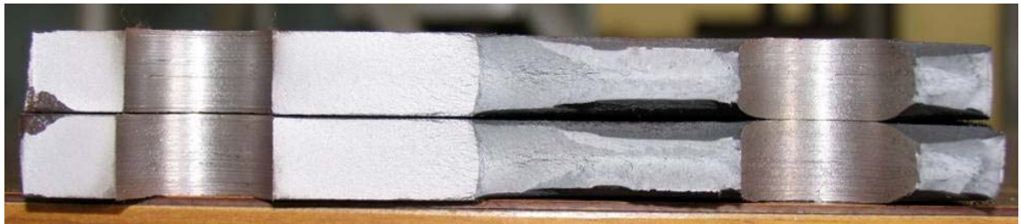
Figure G.6: Cross-Section of A588 - Drilled Hole Plate Specimen at Failure, Drilled with Worn Drill Bit, N=710,415
